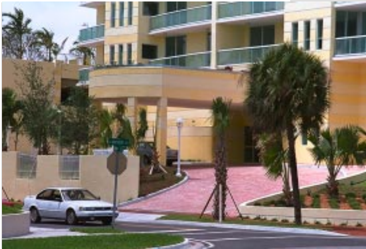
Curb cuts for entry points should be minimized and located on secondary streets when possible.
